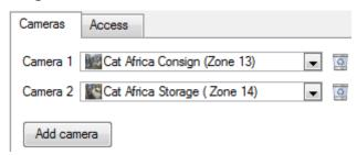
Adding a camera to an object will mean that, whenever there is an event on that object, the recording from that camera will be related to the time and date of the object event, in the Integration database.
